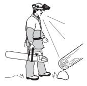
5 Take great care when cutting a tree that is under tension. A tree that is under tension may spring back to its normal position before or after being cut. If you position yourself
